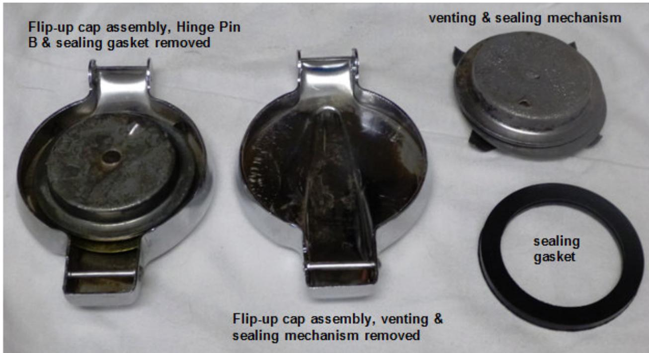
The following picture again shows the chrome flip-up cap, the cap with the venting and sealing mechanism removed, but this time the venting and sealing mechanism is shown from the reverse side. Please note the four spring-steel Anchor Claws that secure the venting and sealing mechanism inside the chrome flip-up cap at about the 2, 4, 8 and 10 o'clock positions (no apology here to the Millennials that never learned analog clock time positions).
